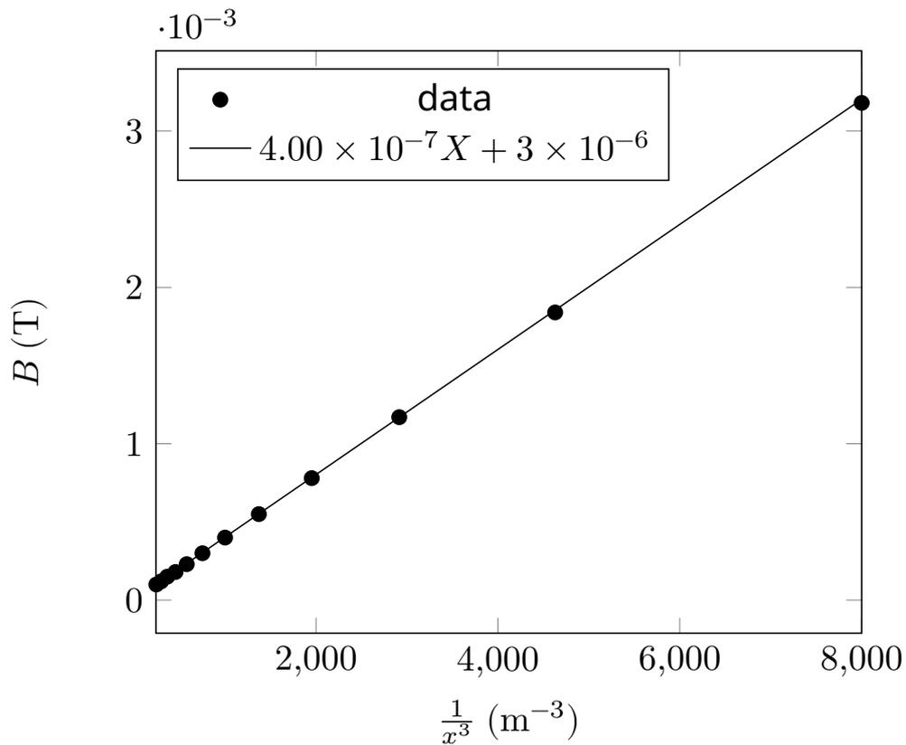
Slope of the graph:  $4.00 \times 10^{-7} \text{ Nm}^2/\text{A}$
