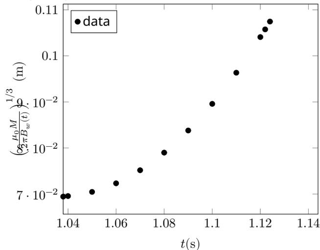
Wooden section is the middle section of the pipe. We have already established in A1 section that the magnet exits the Al section at 1.040 s. We tabulate the data of velocity vs time for this section. Notice that the velocity of the magnet suddenly drops at 1.124 s. At this moment, the magnet enters in the copper section of the pipe and comes under the influence of damping due to the eddy current.
