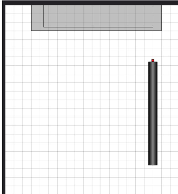
Consider the case when the magnet is at rest at a distance  $x_0$  from the magnetometer origin. The magnet is released along the axis of the pipe. It will start descending through the pipe. In the conducting sections of the pipe, after a brief period of accelerated motion, the magnet will attain a terminal velocity  $v$ , due to the presence of eddy current damping. In this case, the magnetic field  $B_w$  measured by the magnetometer changes with time  $t$  as
