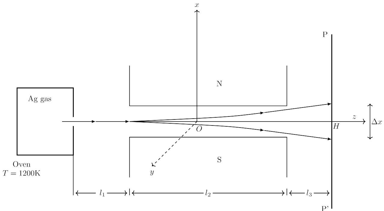
Figure 1: Schematic diagram of the Stern-Gerlach setup.
